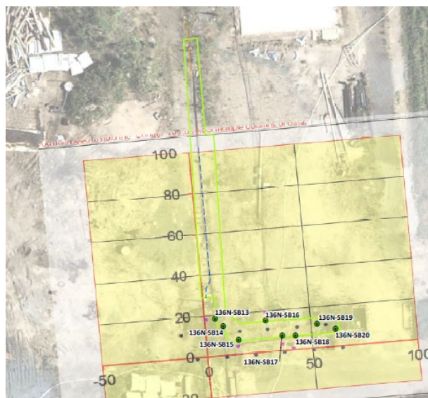
Systematic Random Sampling Locations Central Excavation Area (Terraphase 2024)
